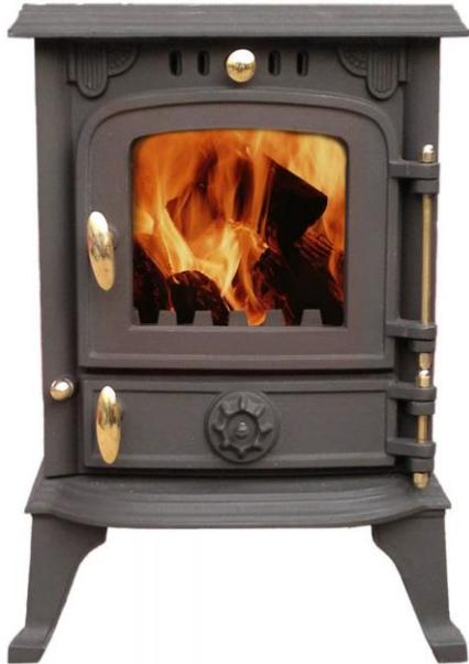
The stove has three air flow controls, one at the top and two at the bottom. Put simply, light the fire with the top slider to the right and the two lower sliders (which can be locked down on their screw threads) open to maximise airflow. When it is going well, push the top slider to the left. The fire will burn about a bucket of coal in an evening.
